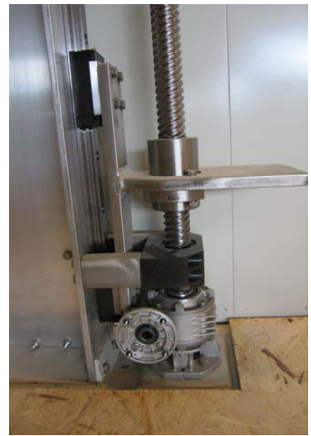
Lifting mechanism inside the container
