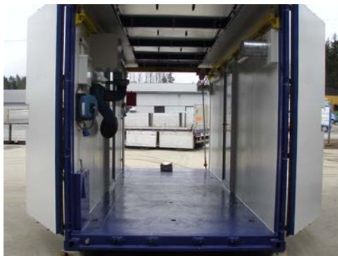
Double doors were installed in each end of the container
