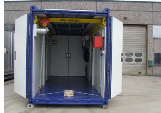
Double doors were installed in each end of the container
